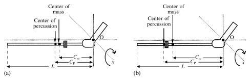
**Figure 3.** (a) A mass attached near to the hand (one-third the length of the rod measured from the rotation point O in the wrist) produces a smaller moment of inertia and a closer center of percussion than (b) a mass attached far from the hand (two-thirds the length of the rod). (Compare the locations of the center of mass and the center of percussion to their locations on the homogeneous rod of figure 1.)
